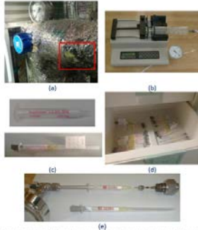
Figure 108. SPA sampling in (a) 100 mL sampling vials or (b) sealed sampling vials (c) 100 mL and (d) 100 mL sample bottles + sample protected by plastic cap + rubber septum ready for storage after sampling (e) SPA samples stored in frozen (200 mL) sample bottles (ready for gasification).
