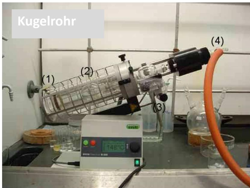
Kugelrohr (German for "ball tube") is a short-path vacuum distillation apparatus
