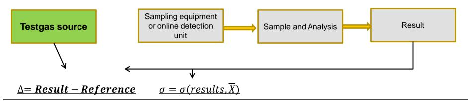
Test procedure 2: a reference sampler or / and an alternative device is synchronous available.
