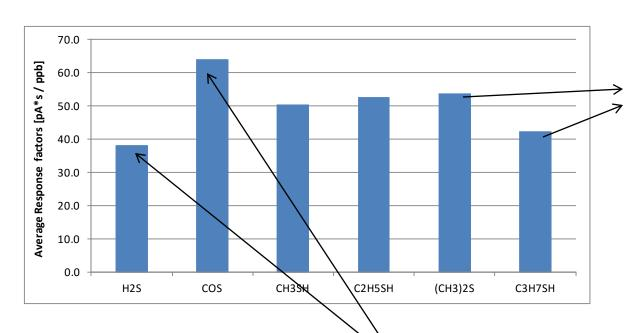
Not all response factors are perfectly equal. It is not clear if the differences across compounds is due to errors in the calibration gas or due to the detector response not being perfectly equimolar.
