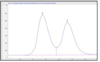
Differences in H<sub>2</sub>S versus COS may be explained in the overlapping peaks (wrong integration), or degradation of H<sub>2</sub>S along the sampling path.
