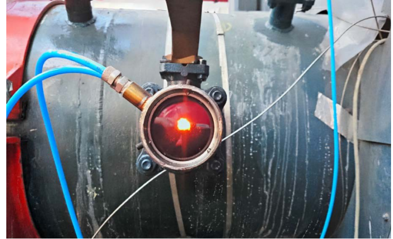
FTIR absorption measurements on the LT-CFB Pyrener gasifier (Kalundborg, DK)
